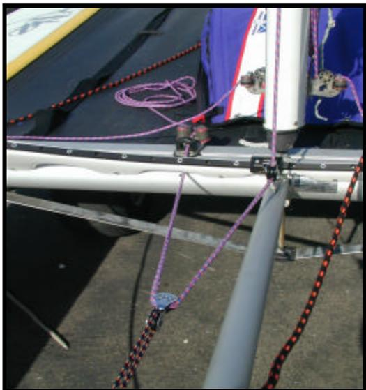
Insert the Aluminum spinnaker pole through the bridle fitting and onto the beam pin. Attach the pole bridle wires to the appropriate tangs on the hulls.
