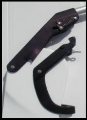
Attach the upper and lower castings to the rudder blades as shown. Adjust the rudder rake by turning the eye screw in or out to the desired location, and tightening the nut.
