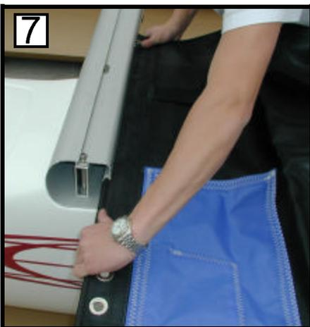
Next, slide each side of the trampoline into the hull tracks (8). Pull slowly and evenly on both sides. NOTE: some models have aluminum trampoline tracks on the hulls.
