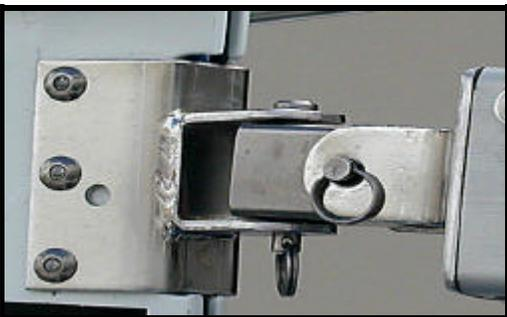
Remove the clevis pin from the gooseneck assembly on the boom, and connect the boom to the bracket on the mast, and pin in place on the mast.
