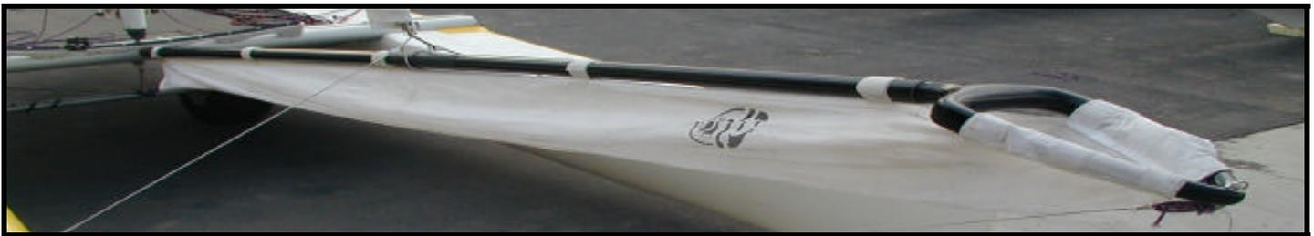
Velcro the snuffer bag onto the pole, and tie the end of the bag to the pin on the pole with the small line on the end of the snuffer bag.
