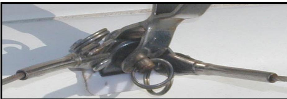
Attach the pole holder to the thin white pole stay wire with the supplied line, and to the pole bridle wires with clevis pins as shown.
