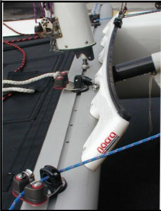
If your boat is equipped with the self tacking jib, the track, and jib sheet controls will be pre-mounted on the forward beam as shown.
