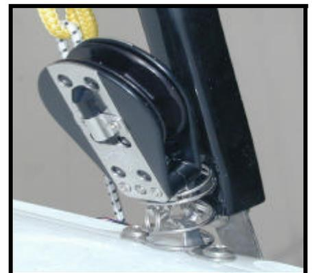
Mount the spin sheet turning blocks on the front beam. Depending on your model, these eyestraps may not be pre mounted– attach them with the supplied rivets approximately 6” inboard of the hull side as shown.
