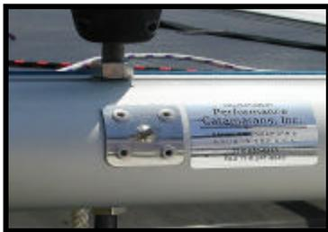
If a spinnaker system is an option on your boat, install the spin pole mounting beam pin in the center of the beam with 4 rivets as shown.
