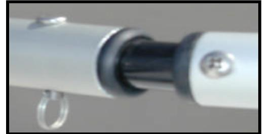
Remove the philips screws from each of the tiller arms, and insert the tiller tie bar. Do not screw it in place yet.
