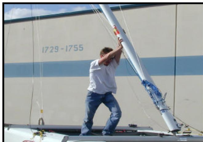
Keep forward pressure on the mast as the second person pins the forestay to the stay adjuster that is attached to the bridle wires. Tighten the rig by putting weight on the trapeze wires and adjusting the pins in the appropriate shroud chain plate holes. Adjust so the mast is raked slightly aft, or straight up. Rake adjustment can be set according to boat handling or wind conditions.
