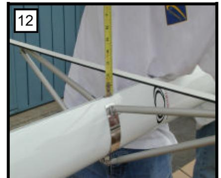
Attach the diamond wires to the mast. Locate the large turnbuckle, and attach one end to the fitting near the base of the mast. Remove the clevis pin from the other end of the turnbuckle and pin the thimble end of the diamond wire to it using the special diamond wire plate clevis pin (13) (Single wire only) and a cotter ring. Pin the forked end of the diamond wire to the upper tang as shown (15).
