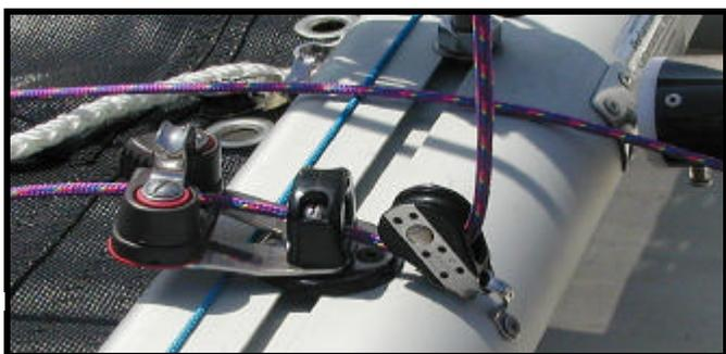
Install the spin halyard swivel cleat onto the beam with the rivets provided on the starboard side of the mast as shown if it is not done so already.
