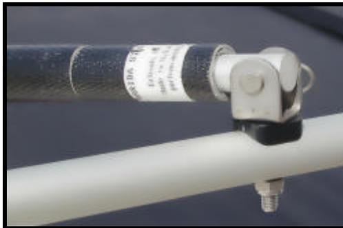
Install the hiking stick on the tiller tie bar using the hardware with the hiking stick.
