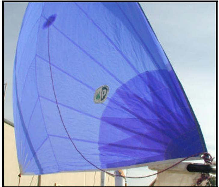
Tie the Tack of the sail onto the snuffer eyes on the front of the snuffer head.
