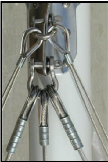
Locate the shrouds and forestay wire or pigtail, and attach them to the large lower hole in the mast hound using the 5/16" bow shackle.
