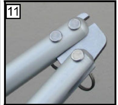
Connect the two arms together with the spreader tip plate and 3 clevis pins on each side as shown (11).
