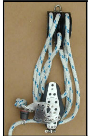
Tie the split tailed end of the traveler line to the two eye straps on the rear beam. Make sure to tie them so the line joins in the middle, allowing the traveler car to be centered. Run the line through the traveler car and cleat. You can tie a stopper knot, or tie the tail end to the mainsheet line.
