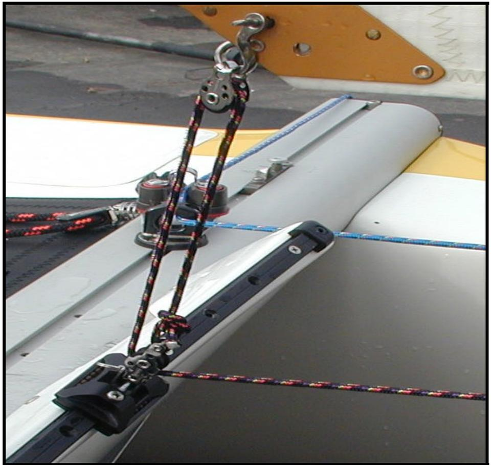
Tie the small line to the airblock floating on the on the large line, and run it back to the becket block on the jib track traveler car, up to the block on the jib, and tie it off on the becket on the traveler car as shown.
