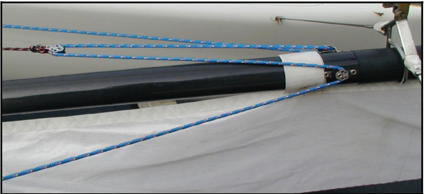
Run the ends of the sheet into the front beam end caps.
