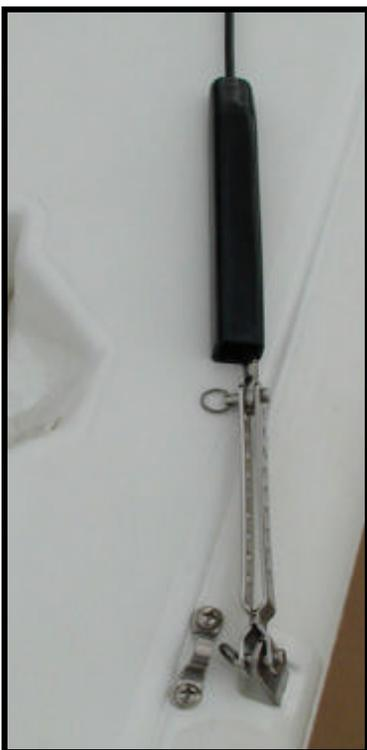
Walk the mast backwards until the base is even with the mast ball. Rotate the mast 90 degrees, and pin the mast base onto the mast ball. You must keep the mast turned 90 degrees until it is vertical to avoid damage.
