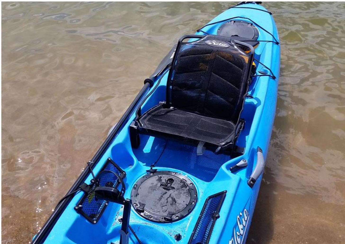
*The Vantage CT. The new elevated mesh seat is incredibly adjustable, front, back, recline, mesh tightness, more.*
