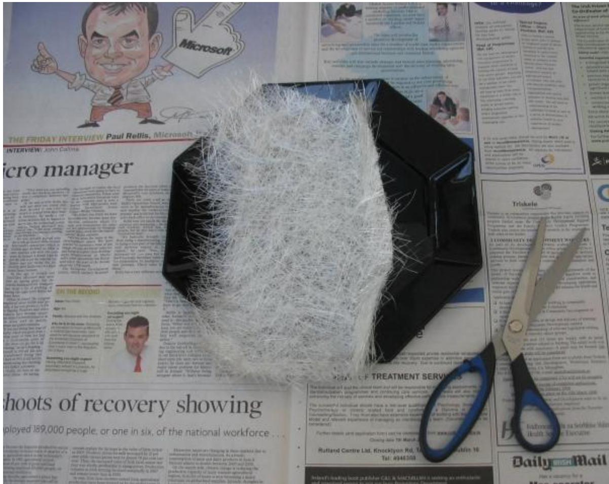
The very small, individual short pieces of glass are in the bowl, epoxy resin is mixed, a bit of glue powder was added to the mix before adding the bits of glass.
