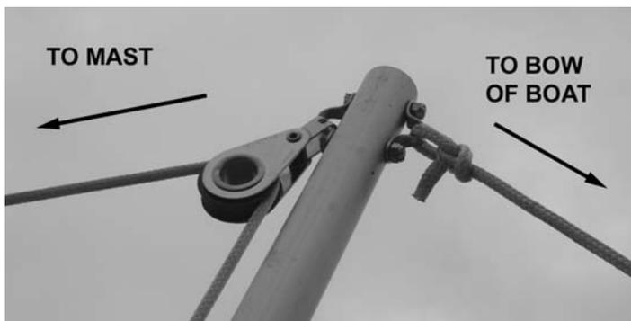
**Pulley and forward line at top end of pole**
