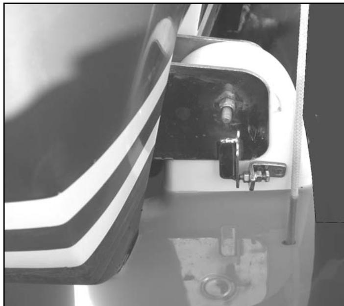
**Rudders secured in the full down position**
